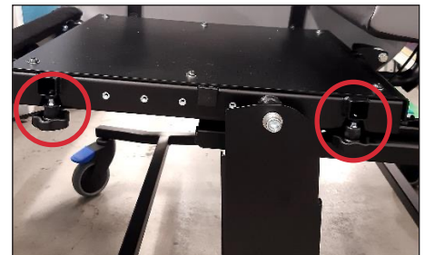
Location of the hand wheels underneath the seat base for seat width and arm removal.
