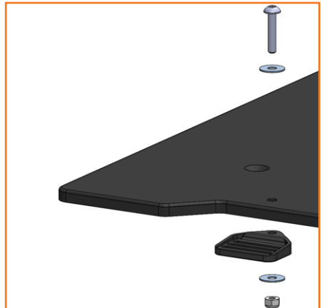
5) Fitting the plastic triple mounting plates.
