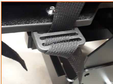
6) Looping the strap through the mounting plate.
