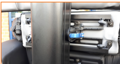
Retrofitting lateral receiving brackets, image shows two sets of receiver tubes being used.
