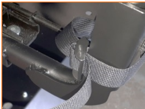
1) Pelvic belt attaches via rear slots.
