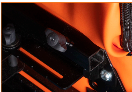
Lateral receiving bracket and hand wheel.
