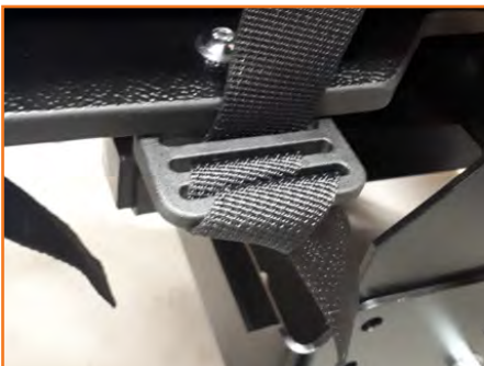
6) Looping the strap through the mounting plate.
