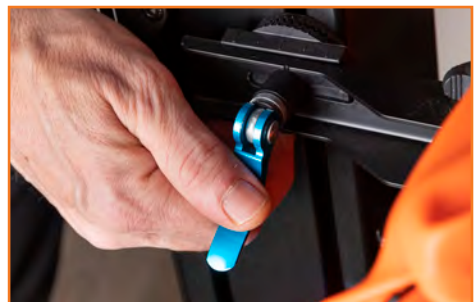
Quick release lever - unlocked.
