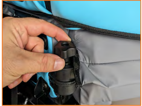
Hand wheel to make lateral wing adjustments.
