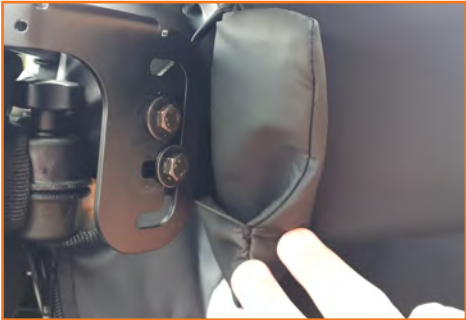
Loosen the two x M6 bolts to reposition the pad.
