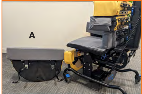
The armrest can be removed completely for side transfers or maintenance.
