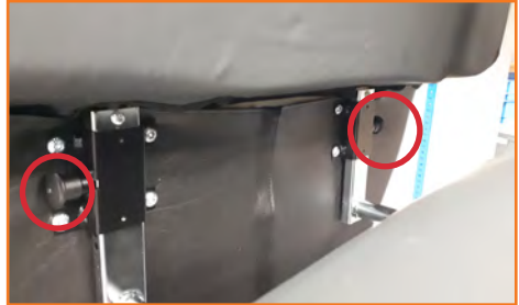
Plunger pins located on the inside of the armrest.
