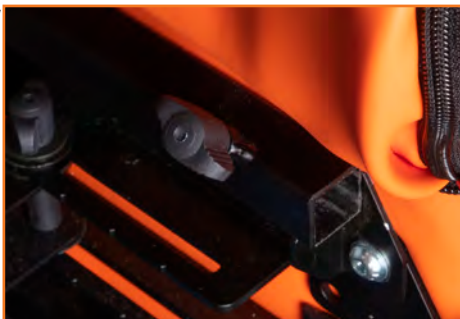
Lateral receiving bracket and hand wheel.
