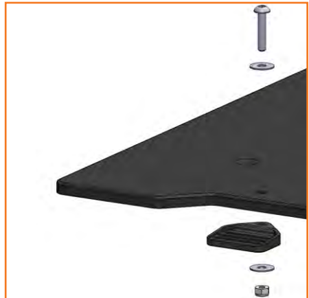
5) Fitting the plastic triple mounting plates.
